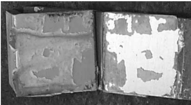
FIGURE 13 Failure surfaces for the L-joint after 30 weeks of immersion.
